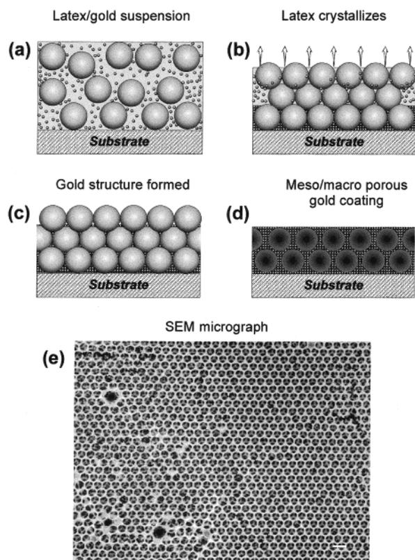
**Figure 1.** Schematic diagram (a–d) of the formation of mesoporous-macroporous gold films templated by colloidal crystals. The porous structure of the resulting material was observed by SEM (e) using a JEOL JXA-840 operating at 20 kV. Scale bar = 1  $\mu\text{m}$ .
